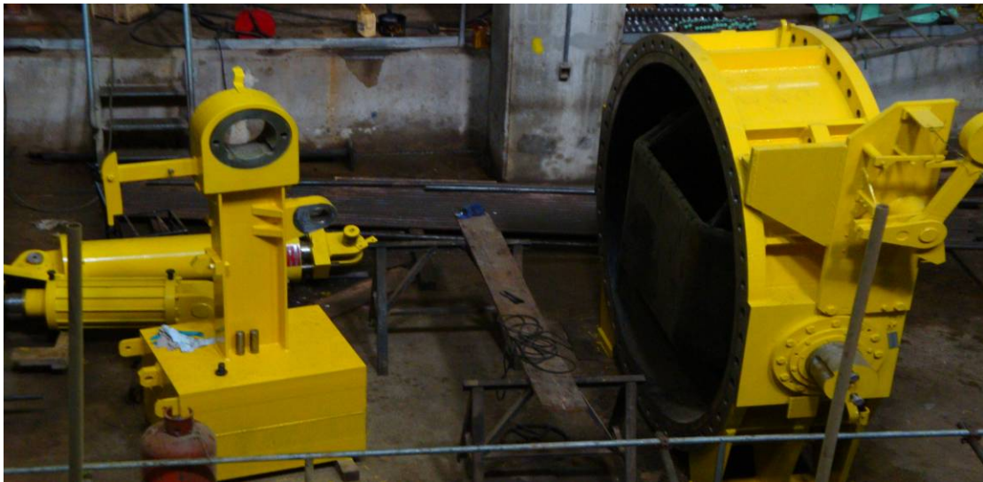
Refurbished parts for turbine 3 stored in the Kajakai power plant in Helmand Province. (Photo by the Office of Inspector General, May 2009.)
