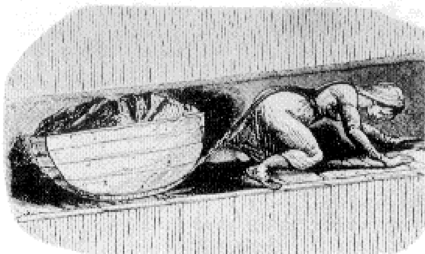
Figure 3.3: A girl pulling a coaltub through the narrow space left by removal of coal from a seam.
