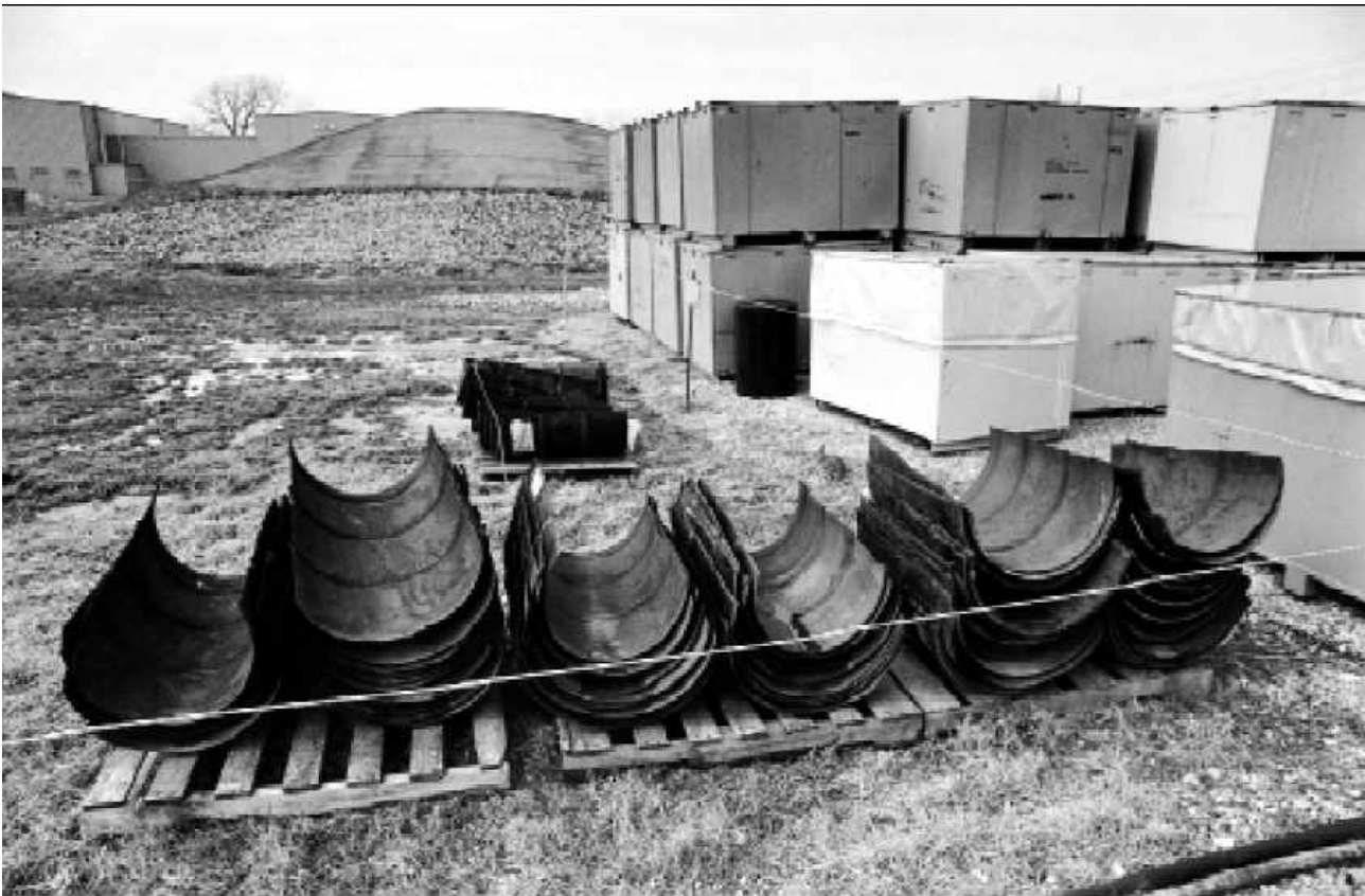
Drums that contain radioactive waste can become radioactive waste themselves, as seen here at the Hazelwood Interim Storage Site outside St. Louis. Source: Linking Legacies.
