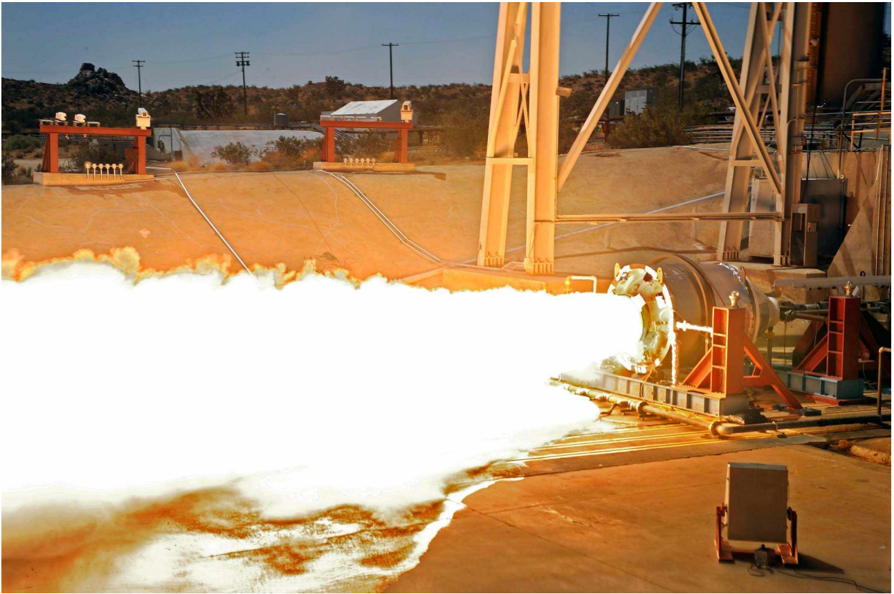
The second stage motor of a Trident 1 C-4 rocket motor was tested at Air Force Research Laboratory Detachment 7 at Edwards Air Force Base July 8. The AFRL testing was part of the Missile Defense Agency's Aging and Surveillance Program and confirmed that the nearly 30-year-old motors remain viable for future MDA missions. (Air Force photo by Ron Fair)
