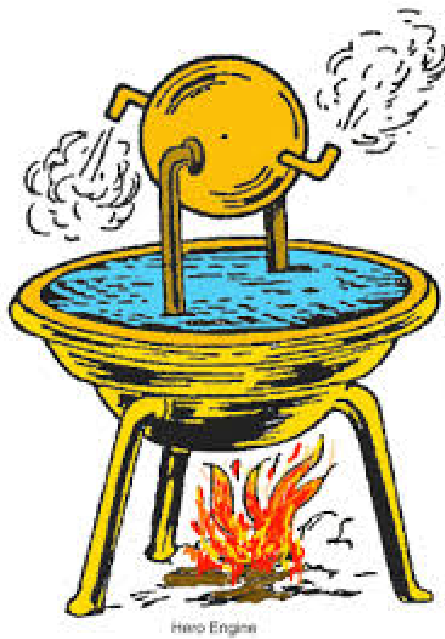
Figure 8.1: A jet-driven steam engine invented by Hero of Alexandria in the 1st century A.D..
