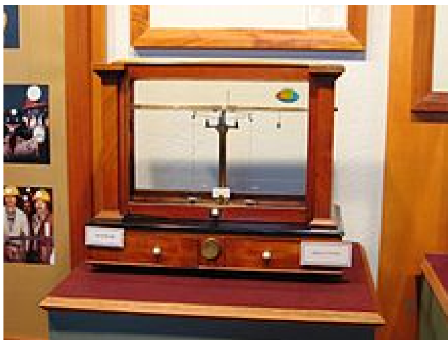
Figure 11.11: One of Joseph Black's important contributions to chemistry was his invention of a highly accurate analytical balance.
